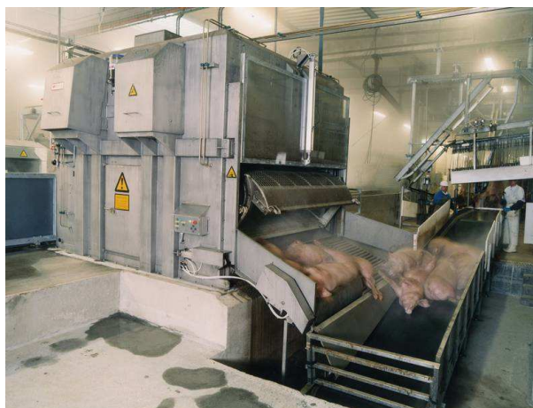
Figure 12. The stunned pigs moving out of the stunner onto the conveyor belt to the 'sticking' point.
