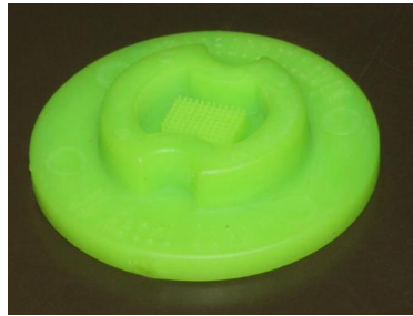
Fig. 4. 96 well micro mould with 400 \mu m diameter wells as used to create the agarose non-adhering cell culture unit
