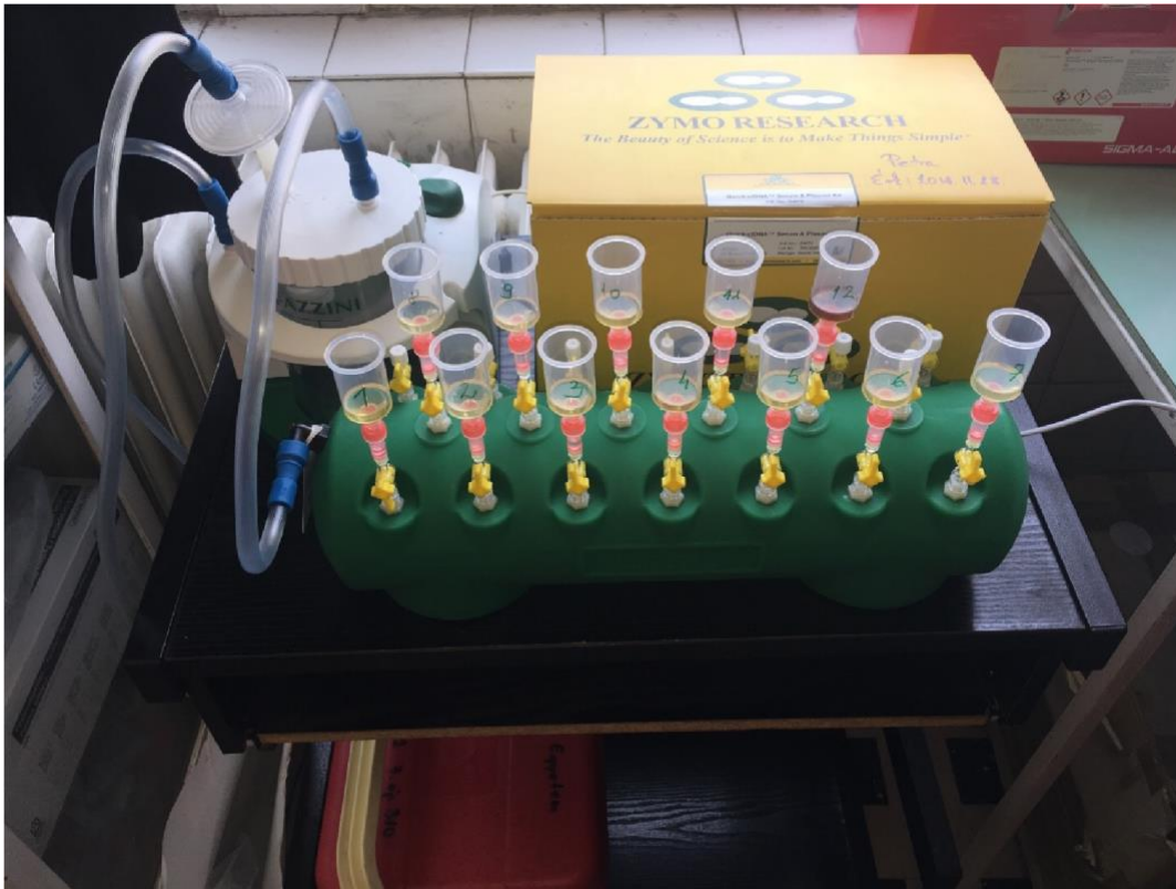
Figure 2- Procedure overview of 12 samples loaded to vacuum vials attached to the vacuum pump. (Department of Animal Breeding, University of Veterinary Medicine Budapest)
