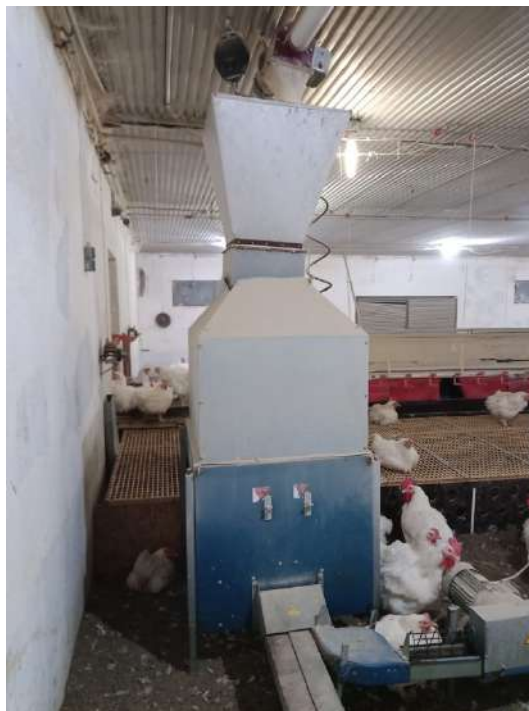
Figure 8 (above) The feeding hopper located at the end of the egg nests for feeding the hens. Note the in-built weighing scales at the top.
