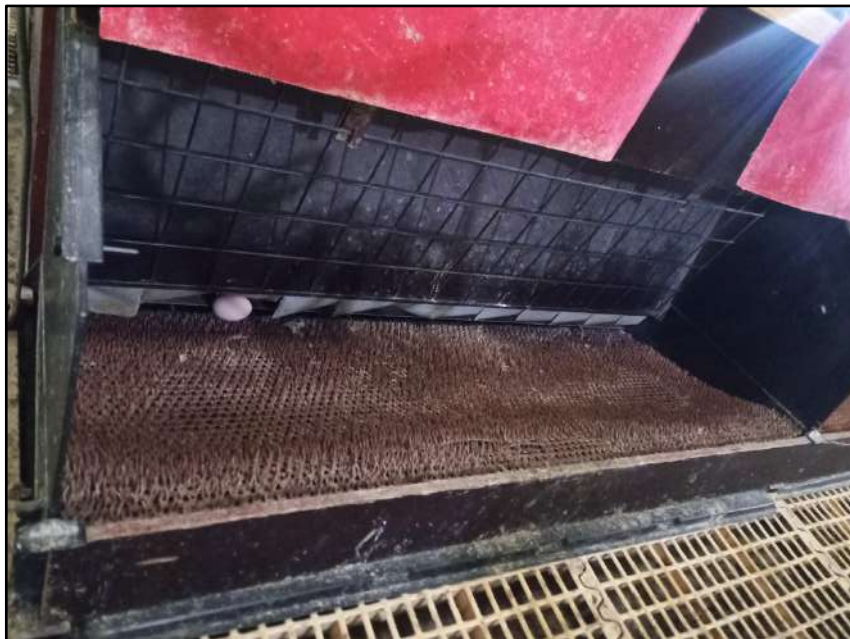
Figure 6 (above) Inside the egg nest. The bottom of the nest contains a carpet to protect the laid eggs. The eggs are then transported by egg belt to the prehall of the barn.
