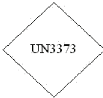
Figure 4: The hazard symbol which should be displayed on the outer packaging of samples (Department of Agriculture Food and Marine, 2014).
