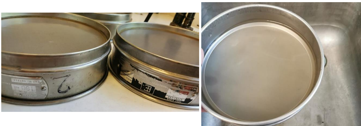
Figure 4 Sieved used for the examinations of faecal samples (picture by author from day of experiment)
