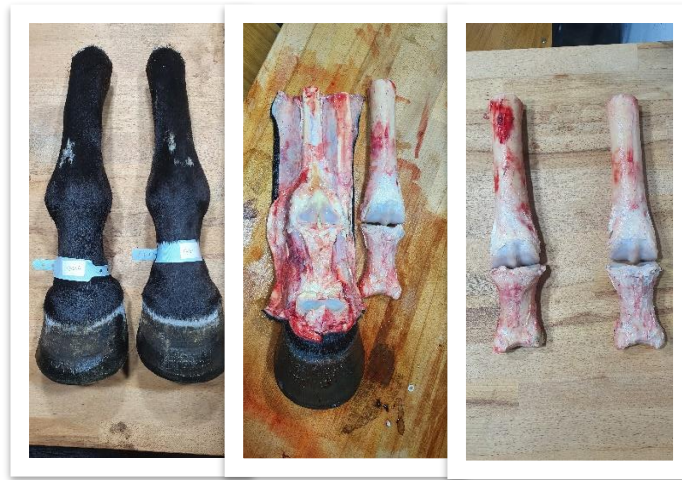
Figure 10- Steps of the removing the soft tissue, melting the labeled legs at room temperature (left), dissection (middle), and bones needed for the experiment (right).
