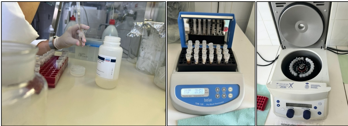
Image 3: Steps during DNA extraction. Pipetting InhibitEx (left), thermo block (central), solution centrifuge (right).
