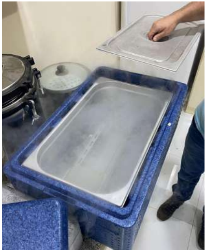
Fig 7.8 Cooling process. Samples are placed in the nitrogen vapor and then plunged into liquid nitrogen for storage.
