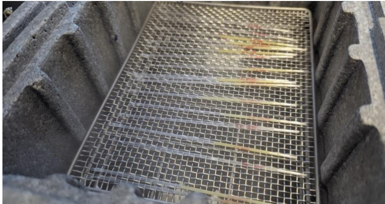
Figure 2: Suspension of the straws 5cm above liquid nitrogen
