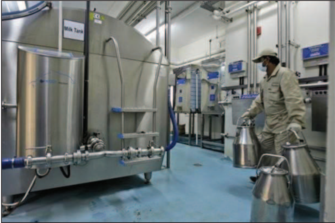
Figure 12 - Cooling tank for temporary storage for camel milk, (Kamran Jebreili/AP)
