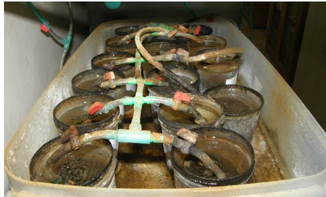
Figure 25: Aerated plastic buckets for individual oligochaete keeping
