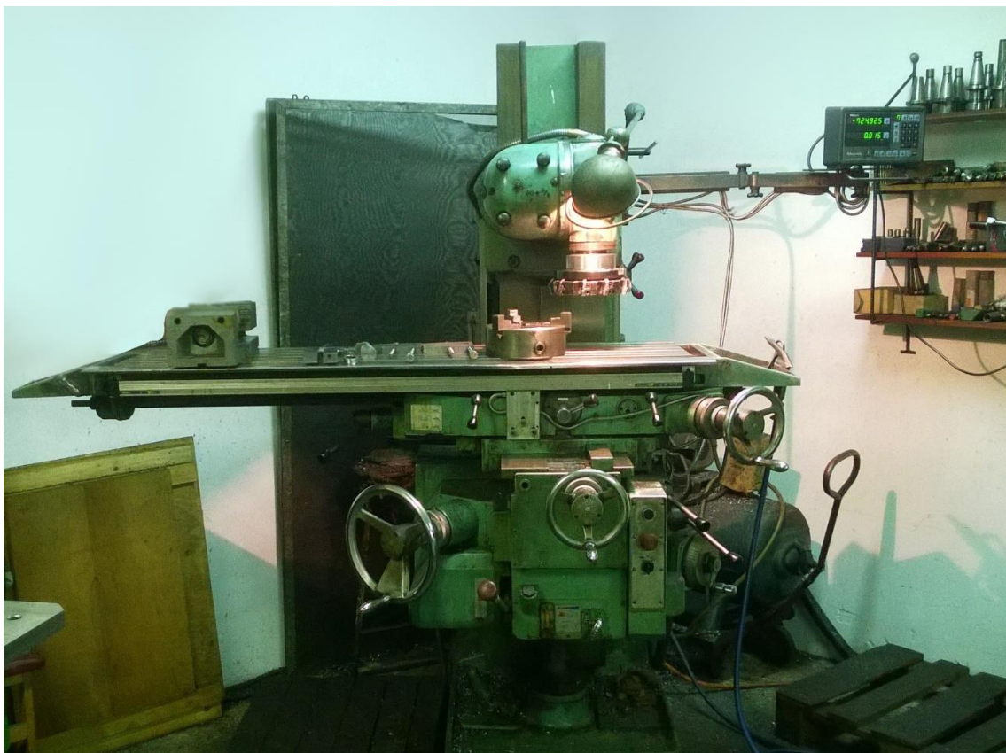
Figure 6. The Dufour universal milling machine which was used in the third pilot study.
