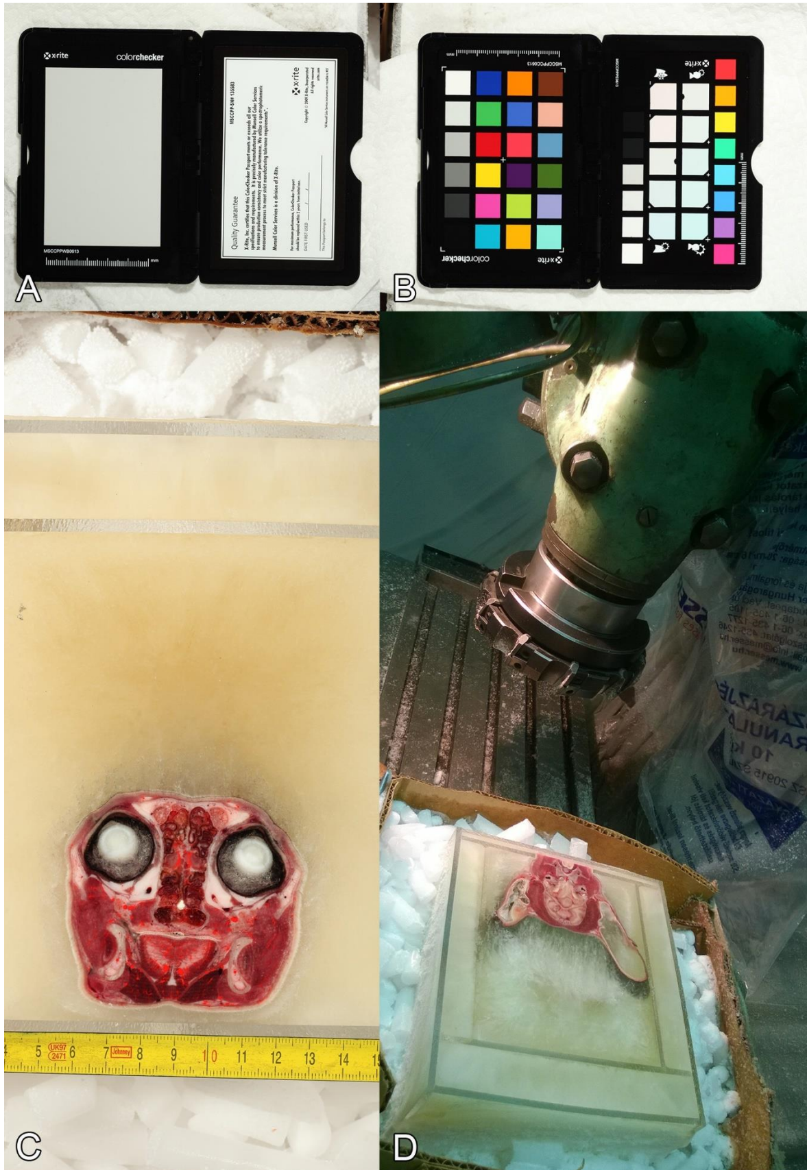
Figure 7. During the cryomacrotomisation process. A, B) Recording the white balance and colour values with a ColorChecker passport. C) The cat head in the frozen gelatin. D) The plexiglass box, surrounded with dry ice pellets during the milling.
