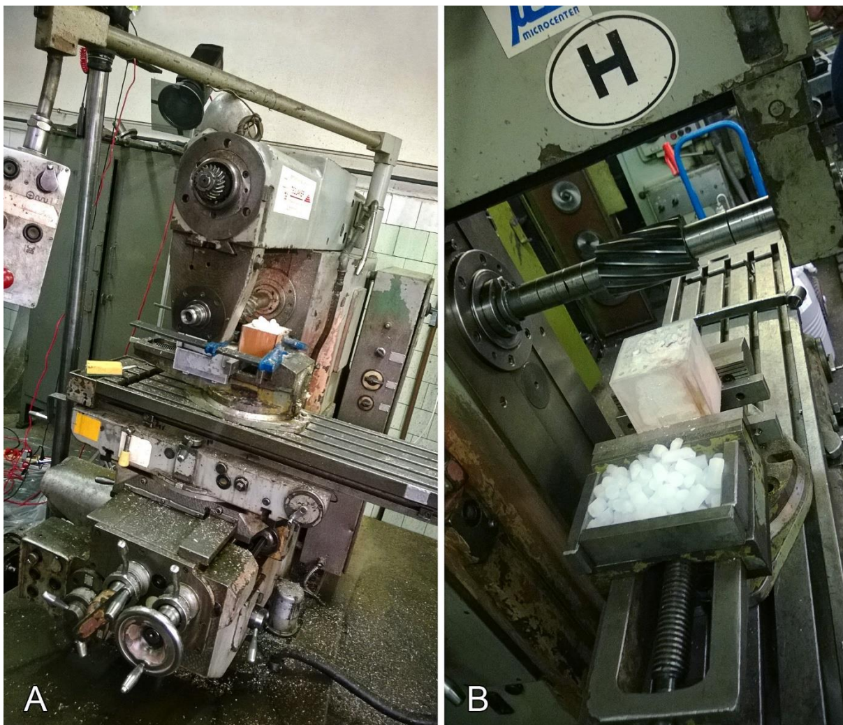
Figure 2. Cryomacrotomisation of a dog head block. A) The JAF0 universal milling machine with the fixed wooden box. B) The rolling mill and the side-cooled embedding box.
