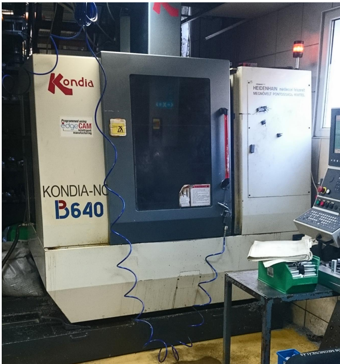
Figure 10. The Kondia CNC milling machine which was used during the fifth pilot study.
