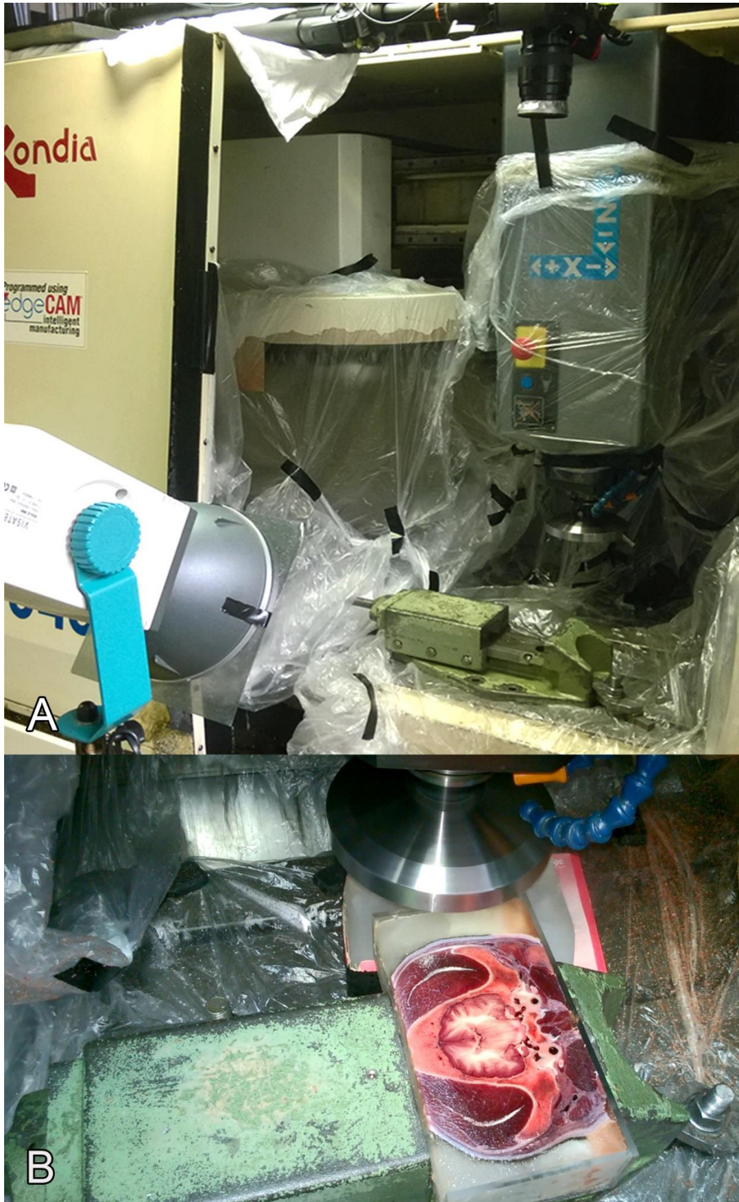
Figure 11. The cryosectioning process. A) Mounting the camera system and isolating the milling area. B) The neurocranial block of the dog in the vise and the flywheel.
