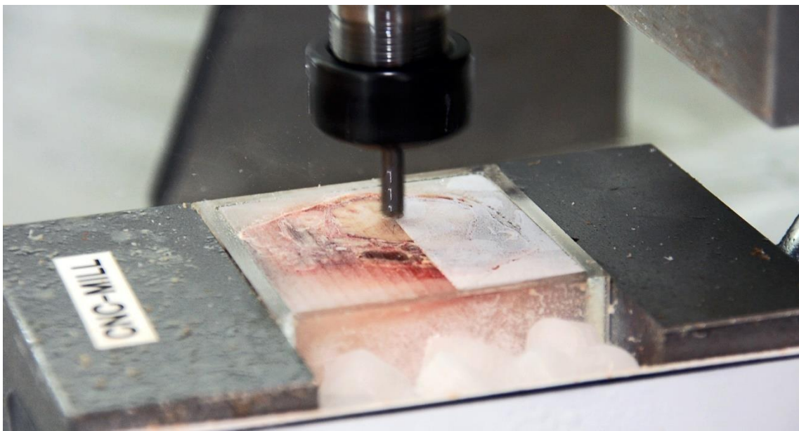
Figure 20. During the cryomacrotomisation of a cat head block with a 2-flute end mill.
