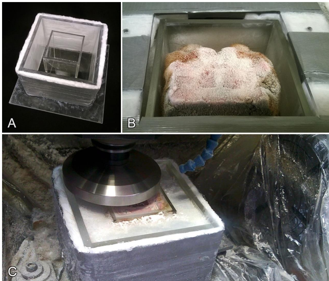
Figure 38. The plexiglass embedding box during the different stages of the procedure.
